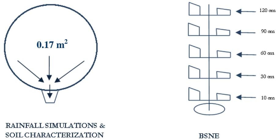
Figure 4 Experimental set-up
