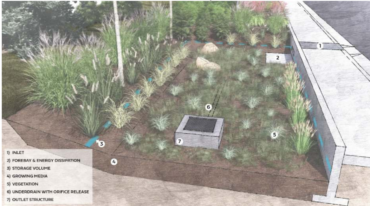
Figure BR-1. Bioretention System Components
