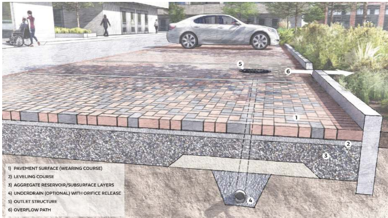
PPS-1. Permeable Pavement System Components
