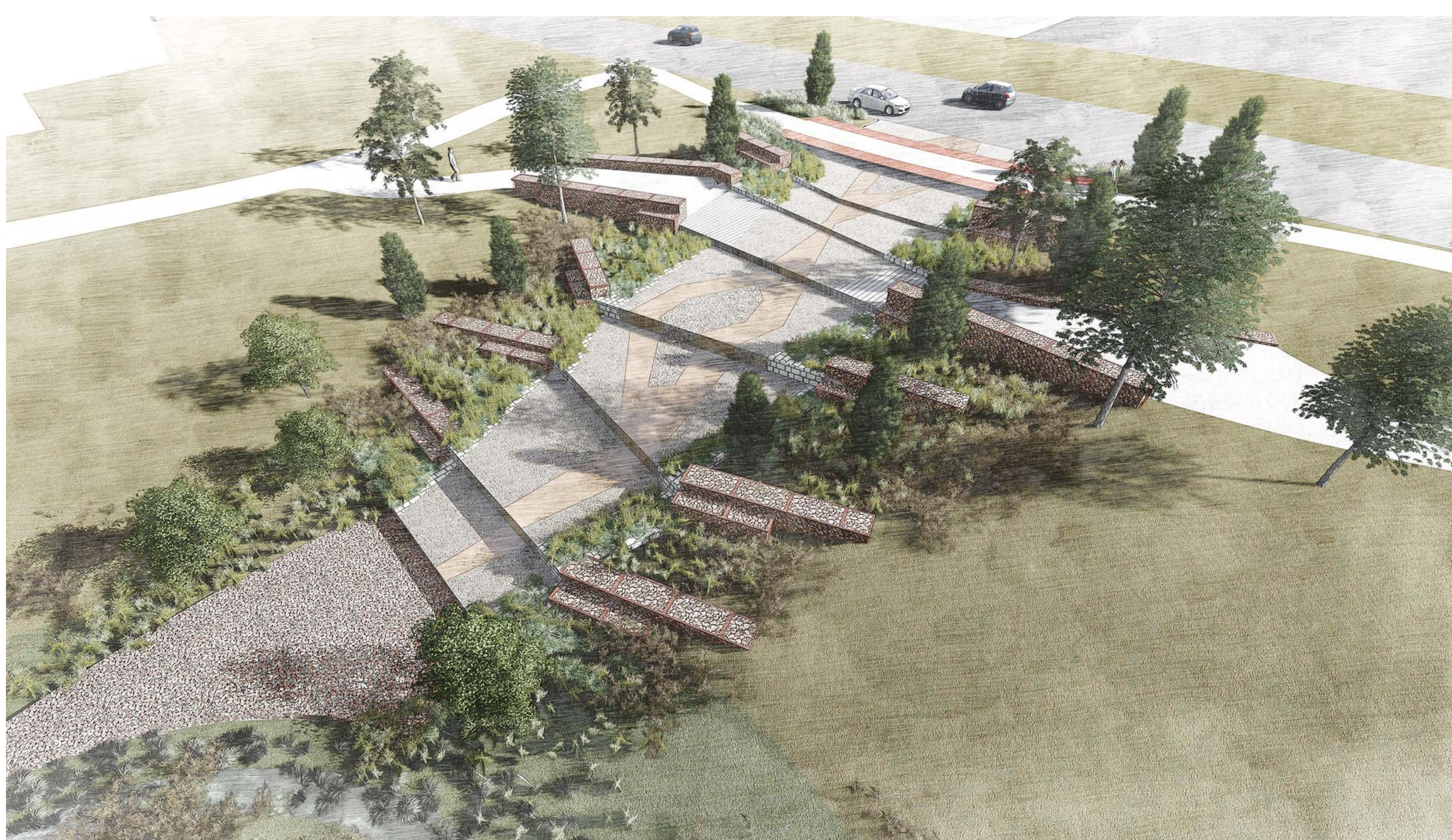
VIEW 1: Bird's-eye rendering of drop structure design showing gabion walls, paving pattern, box culvert crossing, forebay, and vegetation.
