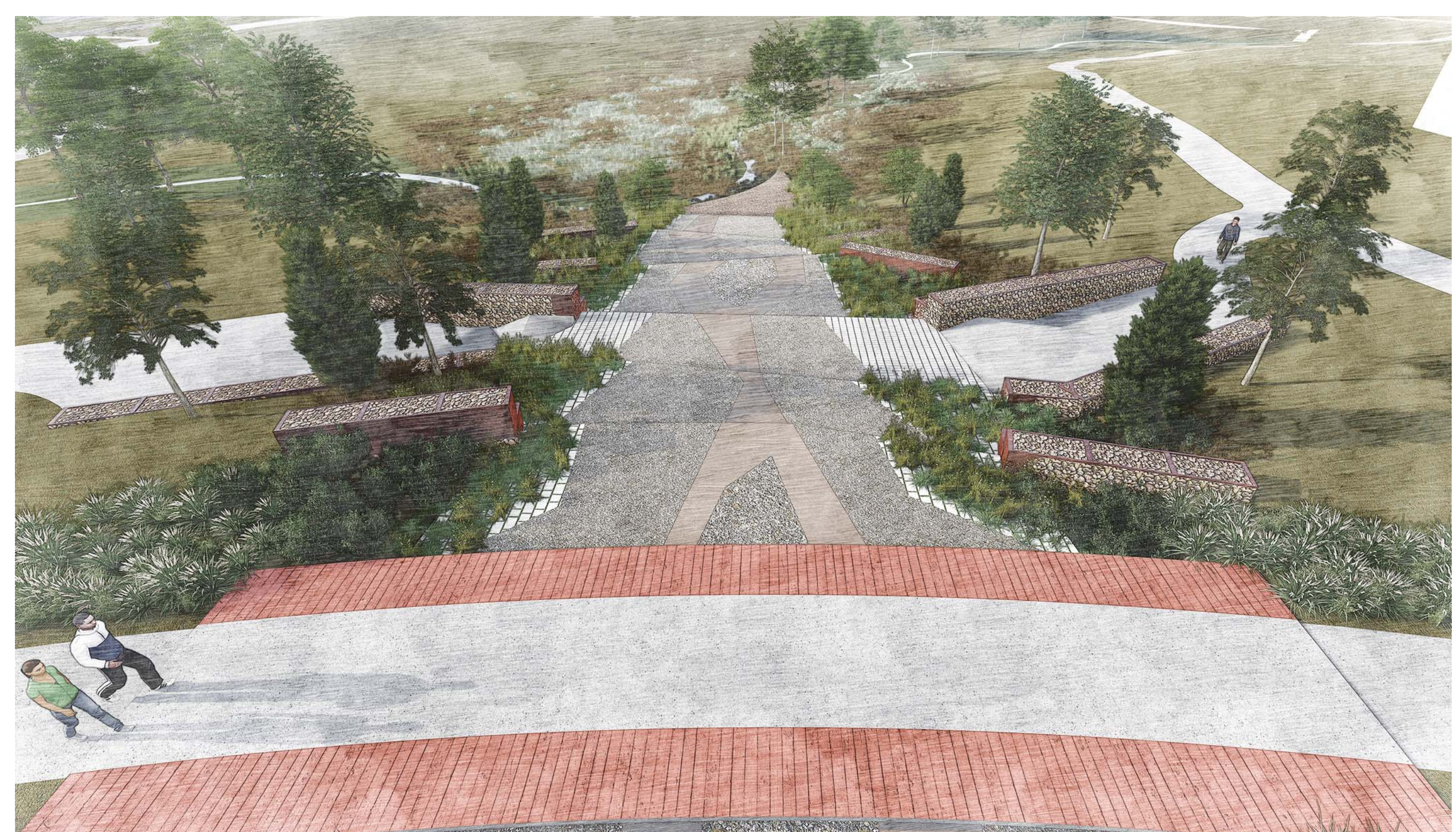
VIEW 2: Rendering of drop structure design showing box culvert crossing, gabion walls, paving pattern, and trickle channel beyond.
